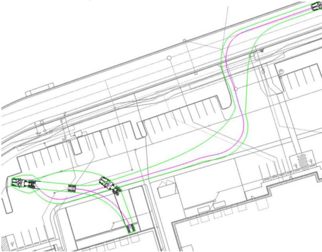
Figure 3: WB-67 Tractor/Trailer Truck Exit
