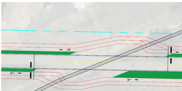
Figure 9: Recommended Rail Crossing
