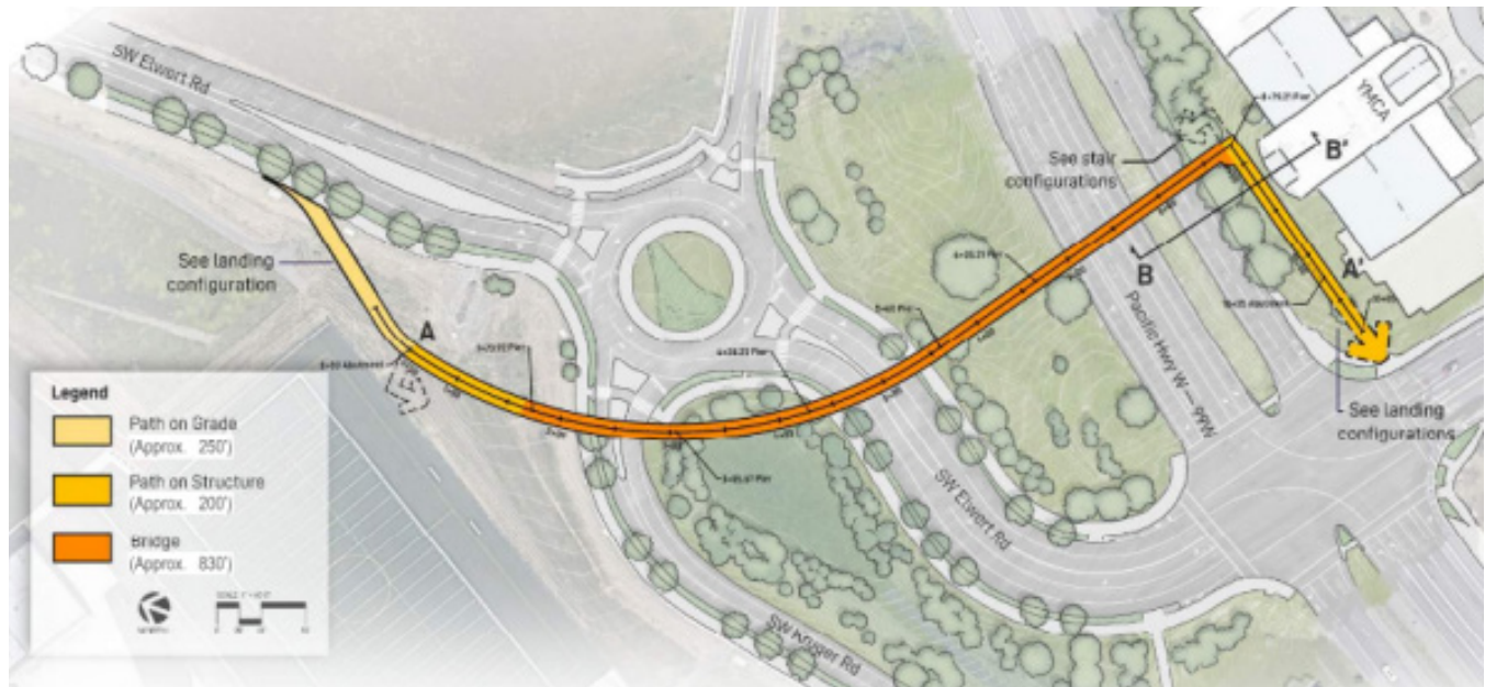
Figure 18. Pedestrian Overcrossing Alignment
