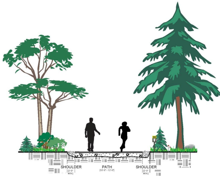
Figure 1 – Typical cross-section for a shared use path
