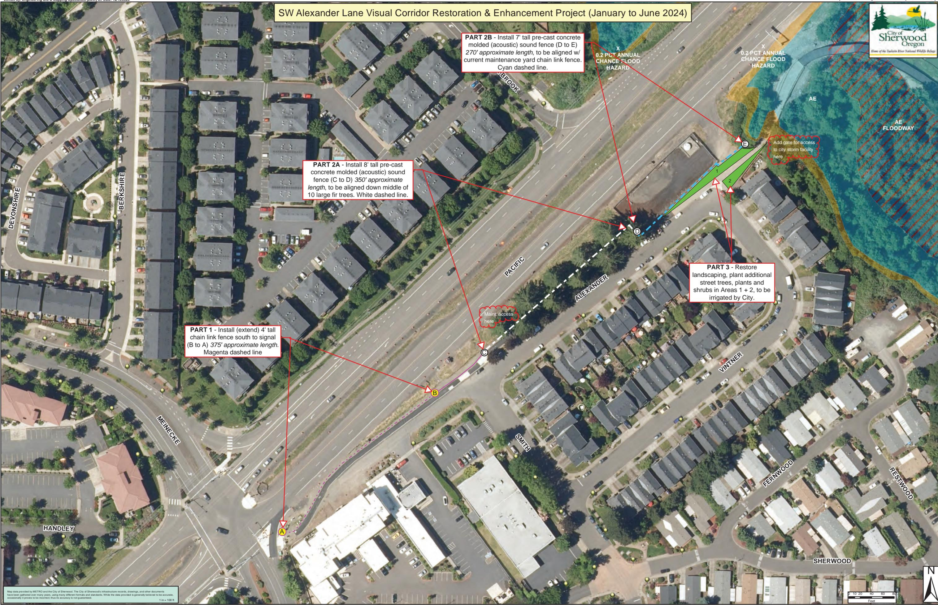
**PART 2B** - Install 7' tall pre-cast concrete molded (acoustic) sound fence (D to E) 270' approximate length, to be aligned w/ current maintenance yard chain link fence. Cyan dashed line.
