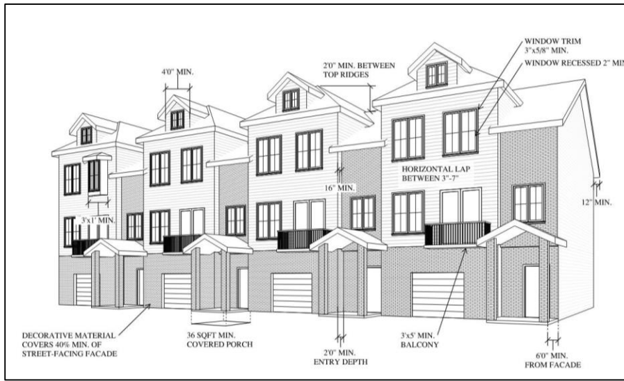
Figure 8. Example of Detailed Design -Townhome (2 elements required)
