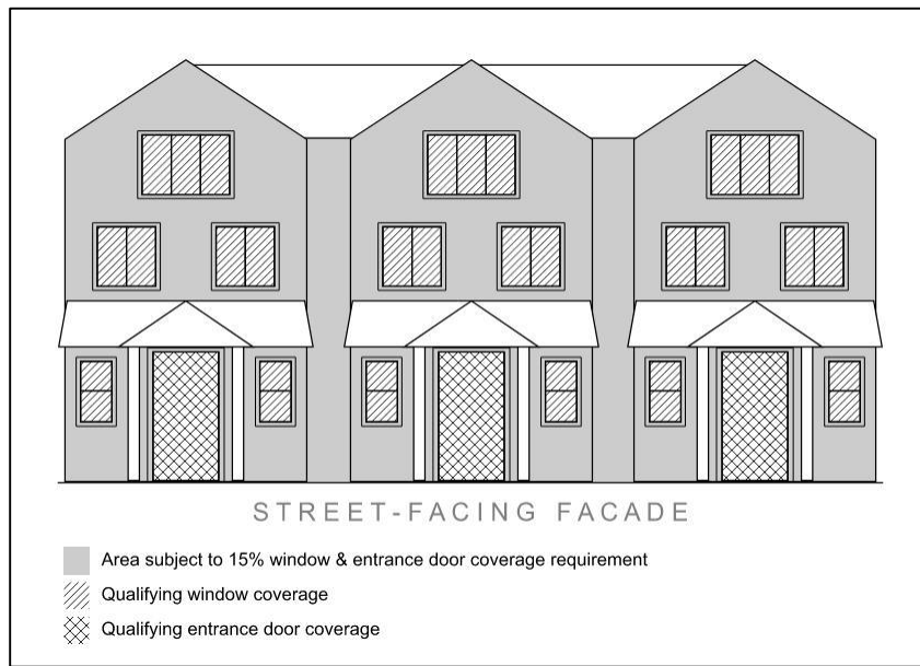
Figure 6. Window Coverage Calculations
