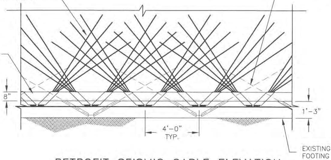
**RETROFIT SEISMIC CABLE ELEVATION**
