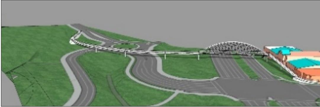
The tall arch main span is a materially efficient and cost-effective structural type, while the twin girder approach span is slightly less so. This bridge option features a signature arch form at the main span across Hwy 99W accompanied by a visually quiet and simple approach span.
