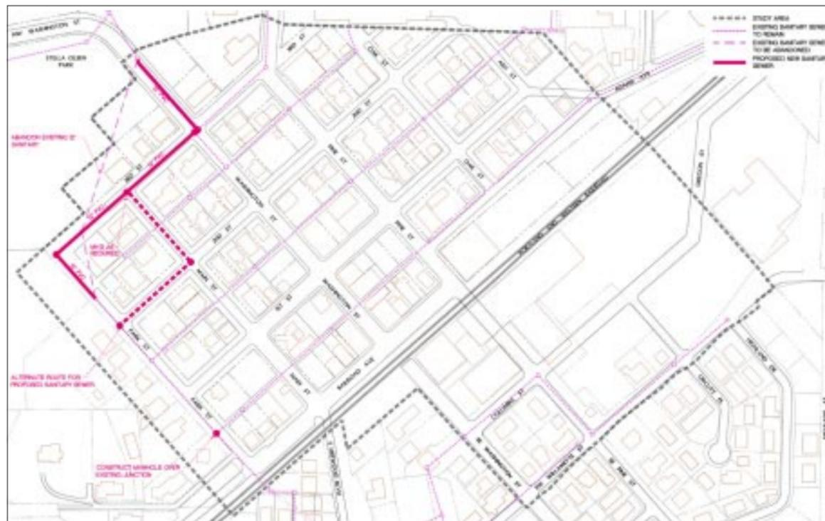
Sanitary sewer reconstruction/rehabilitation plan
