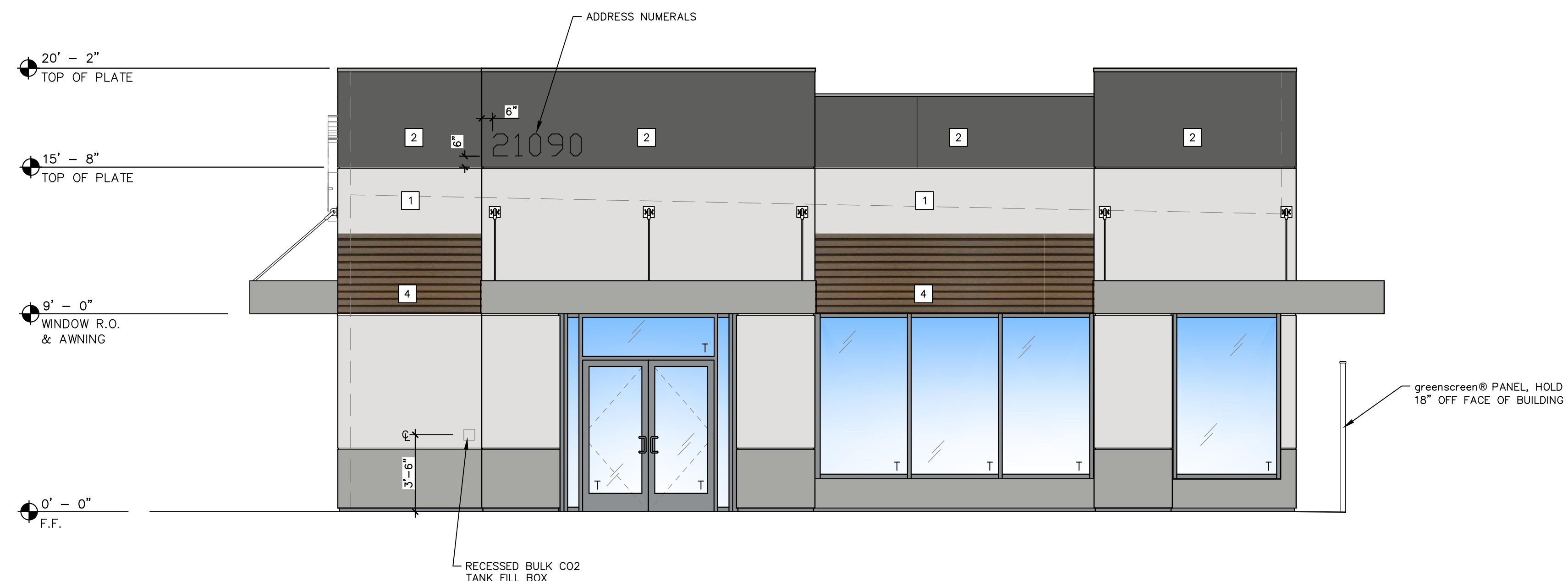
NORTH ELEVATION - FACING SW PACIFIC HIGHWAY SCALE: 1/4"=1'-0"
