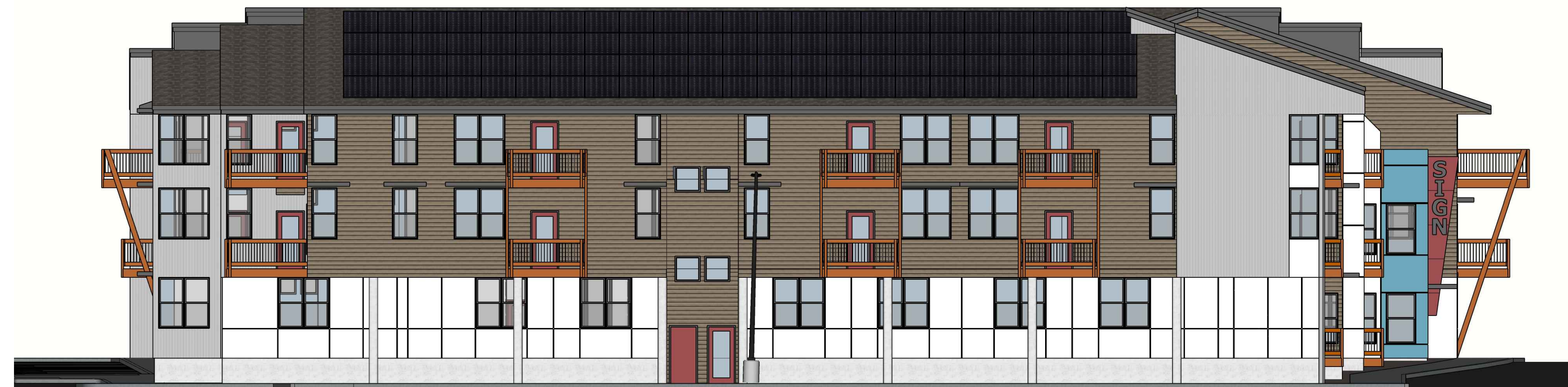
2 WEST ELEVATION - METAL SIDING A3.2a SCALE: 1/8" = 1'-0"
