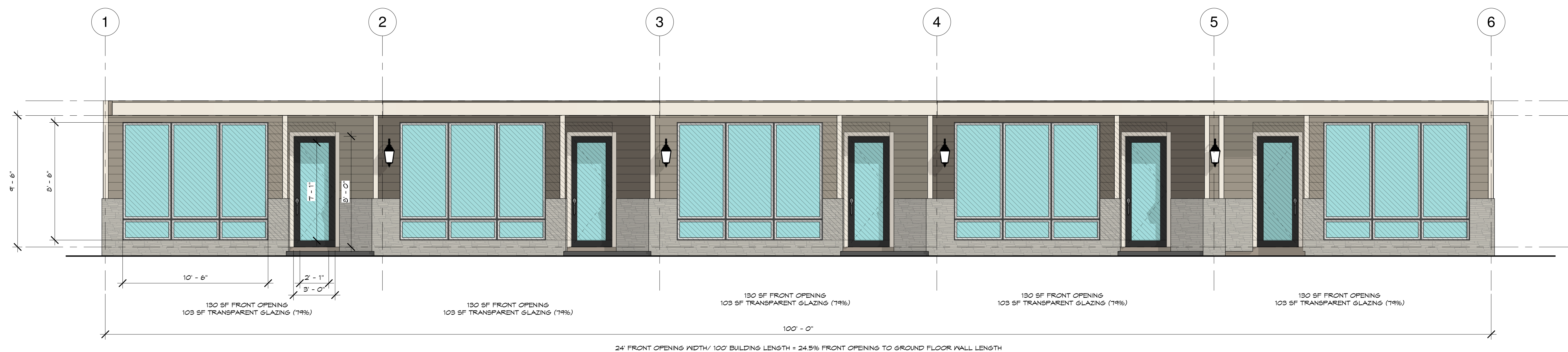
North Elevation Ground Floor Glazing 1/4" = 1'-0"
