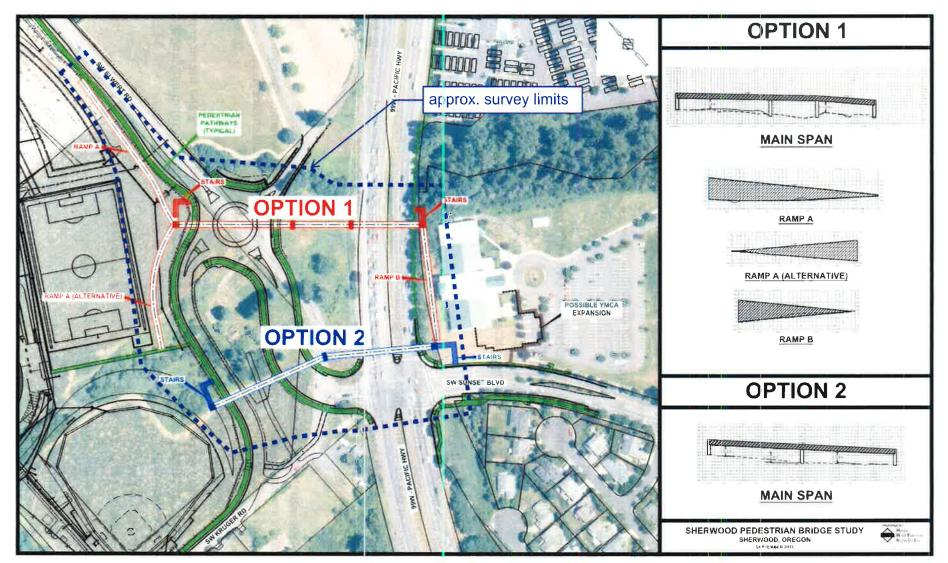
Figure 6: Alignments Used for Cost Estimates of Pedestrian Overcrossing
