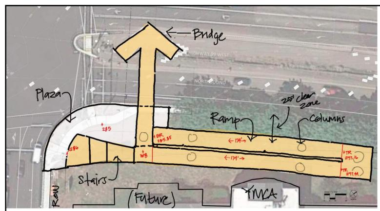
plan view \_\_\_\_\_ massing perspective
