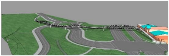
The material efficiency of the Bowstring Truss is lower than that of the tall arch, resulting in slightly more material required and additional cost. The net effect is the appearance of a single, undulating structure along the full length of the bridge alignment at a more modest structural height than the High Arch option.
