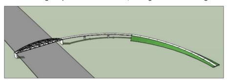
DaVinci Truss: The DaVinci Truss spanning Hwy 99W uses a staggered kingpost and crossed tension
