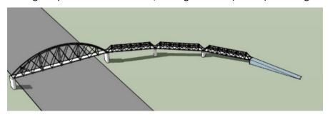
• **Bowstring Truss:** The primary span across Hwy 99W is a twenty-foot-tall through-truss structure with a curved upper cord, giving it a characteristic bowstring form, and a pedestrian deck running through the middle of the truss itself. This structural type is not as tall as the High Arch option (1:10= height: span), making it less efficient and requiring more steel or wood. The shorter approach spans to the west of the highway could be tied arches, through trusses or twin girders (shown).
