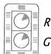
TYPE 8 Ramp Meter Only
