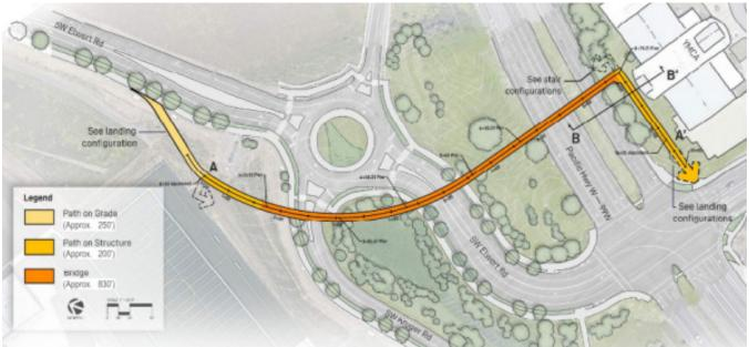
Figure 18. Pedestrian Overcrossing Alignment
