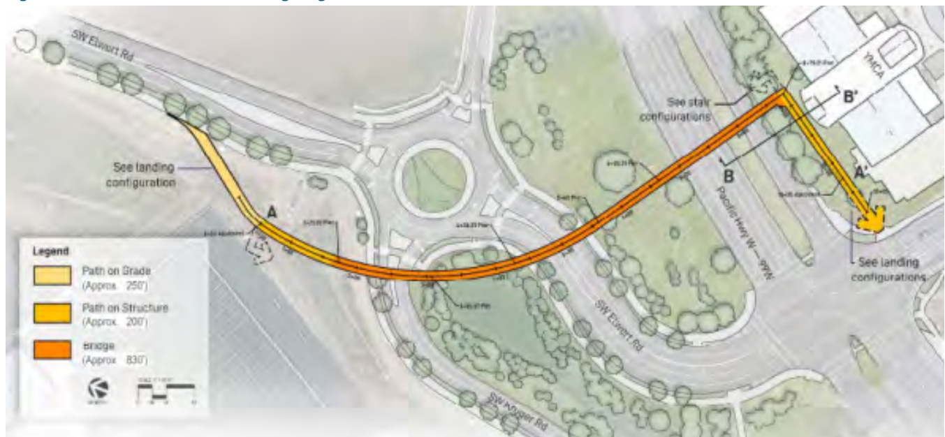
Figure 18. Pedestrian Overcrossing Alignment
