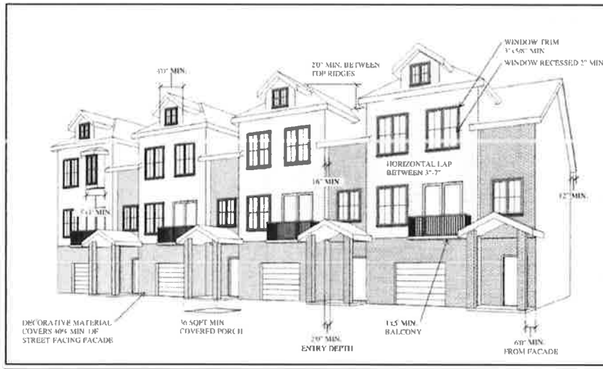
Figure 8. Example of Detailed Design -Townhome (2 elements required)
