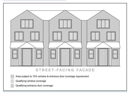
Figure 7. Example of Detailed Design – Single Detached (5 elements required)
