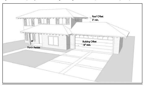
Figure 8. Example of Detailed Design -Townhome (2 elements required)
