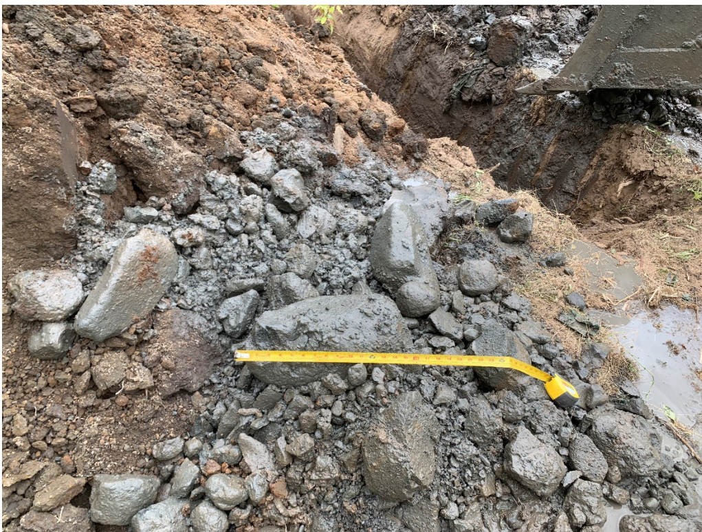
Photo 2. 16-inch Diameter Boulder within Coarse-grained Missoula Flood Deposits
